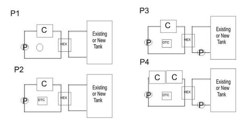
C: Collector, P: Pump, HEX: Heat exchanger, DTC:differential temperature controller
